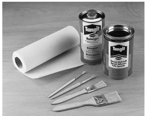
Fig. 3: Solvent cementing equipment
