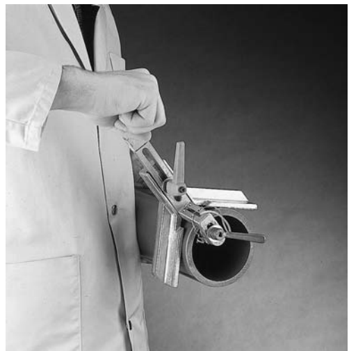
Fig. 2: Chamfering the pipe
