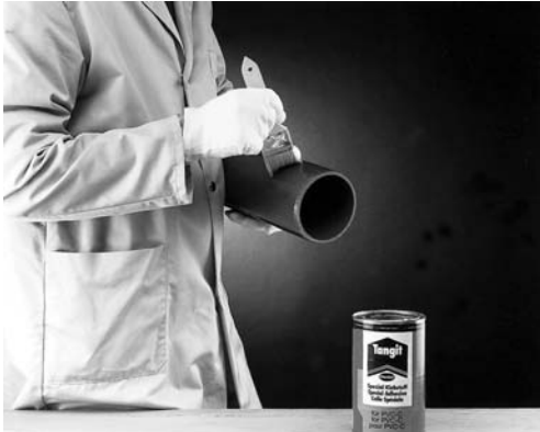
Fig. 6: Applying the cement
