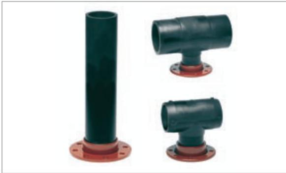
**Draw-Lock transitions between PE and metal flanges.** Draw-Lock is a very compact solution with end-load resistance for integrating metal-flanged fittings like valves and hydrants in PE pipe systems.
